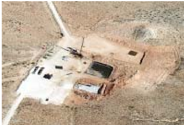
A typical oil well pad in southeastern New Mexico. An average of five acres will be cleared for each well pad constructed on Otero Mesa. Photo courtesy SkyTruth.
